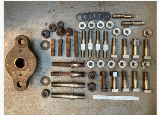
Replacement bolts, nuts and studs made in our workshop.
