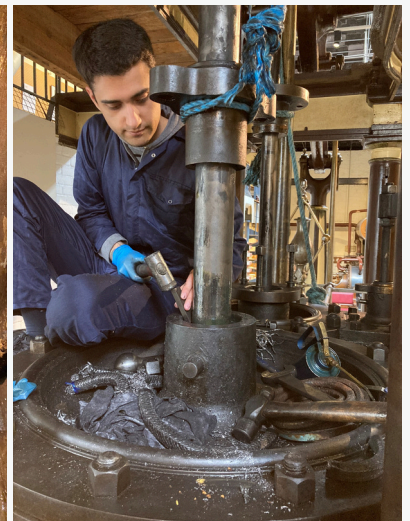
Saeid replacing the steam packings on The Easton and Amos Engine.
