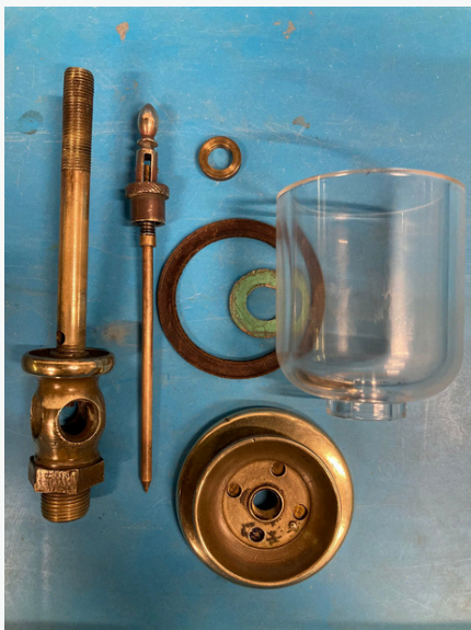
Figure 14: dismantled and refurbished oiler to Waddon engine
