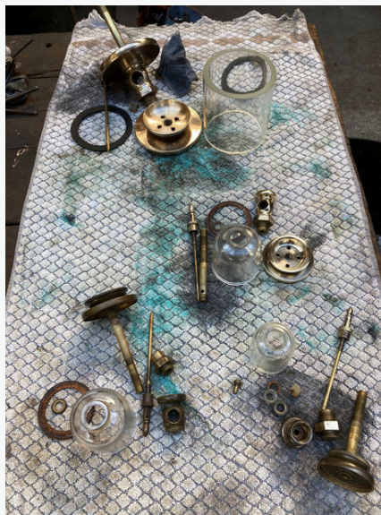
Figure 15: Waddon lubricator parts being cleaned up
