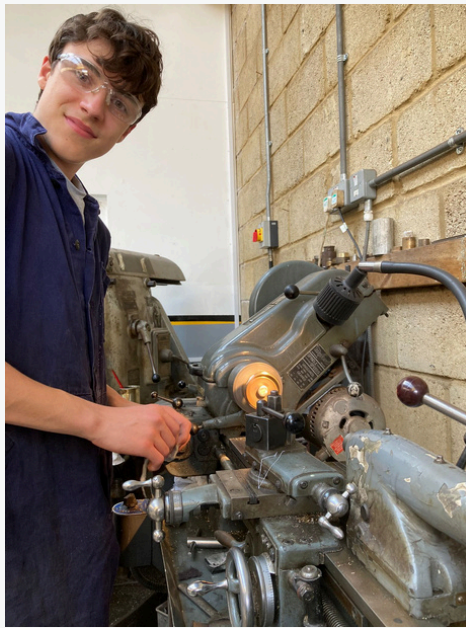
Figure 18: Joe Ellis using lathe to clean lubricator parts for Waddon engine
