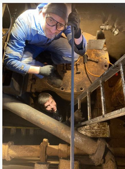
Figures 1 & 2 & 3: air pump dismantling, unbolting air pump top cover, removing air pump piston
