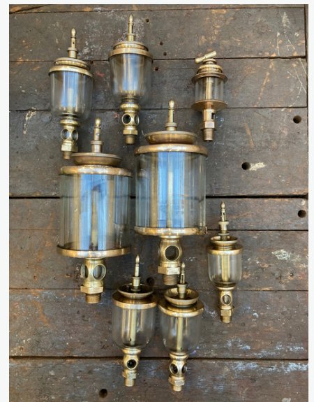
Figure 16: refurbished and polished lubricators ready to refit on Waddon engine
