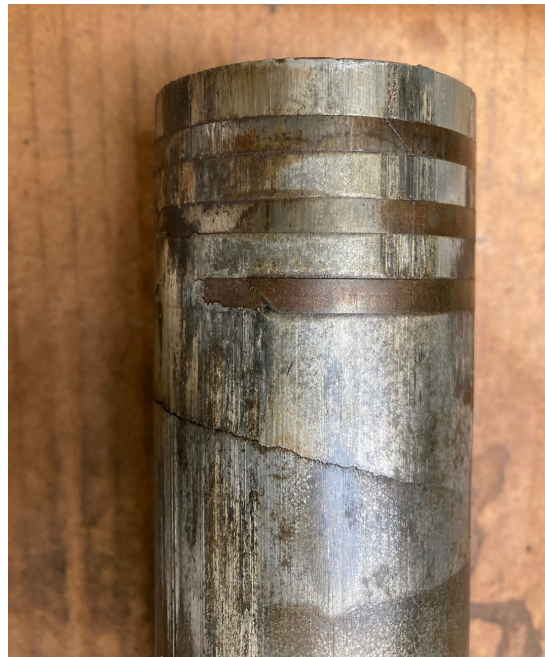
A close up of the cracked piston from the Allen Diesel engine
