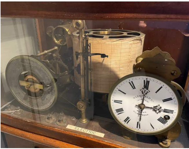
Close up of the electric reservoir level meter, which has moved from the Steam Hall's mezzanine.
